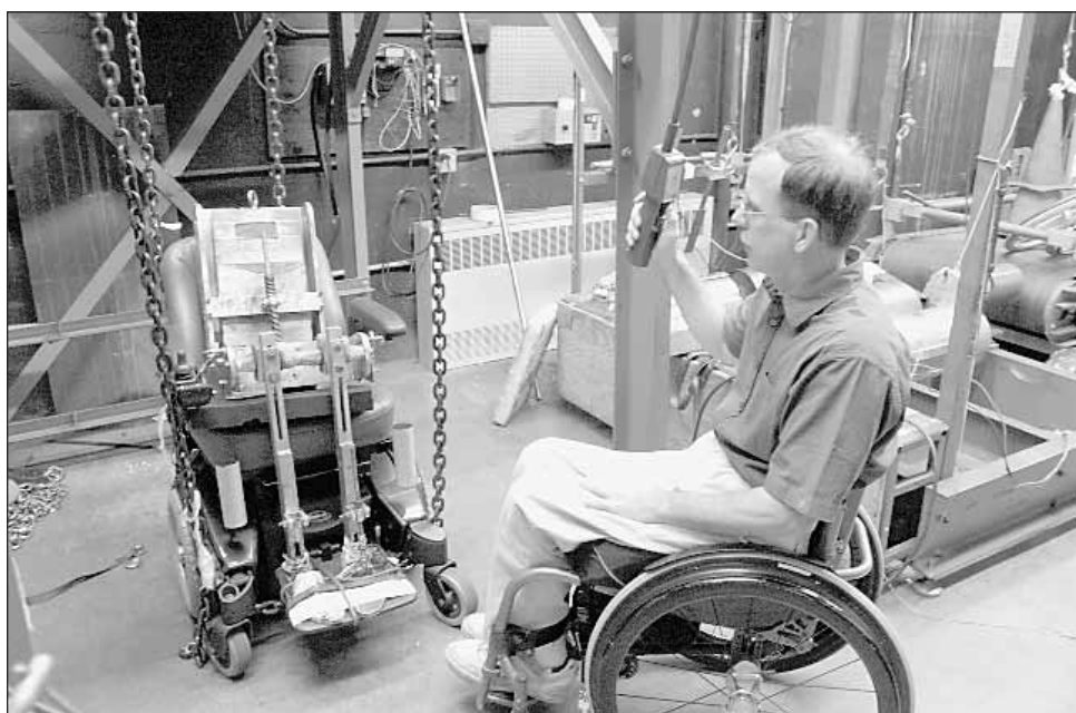
Dr. Rory Cooper checks a new wheelchair by repeatedly dropping the wheelchair carrying a dummy weighing over 300 pound for ANSI/RESNA and ISO standards.
